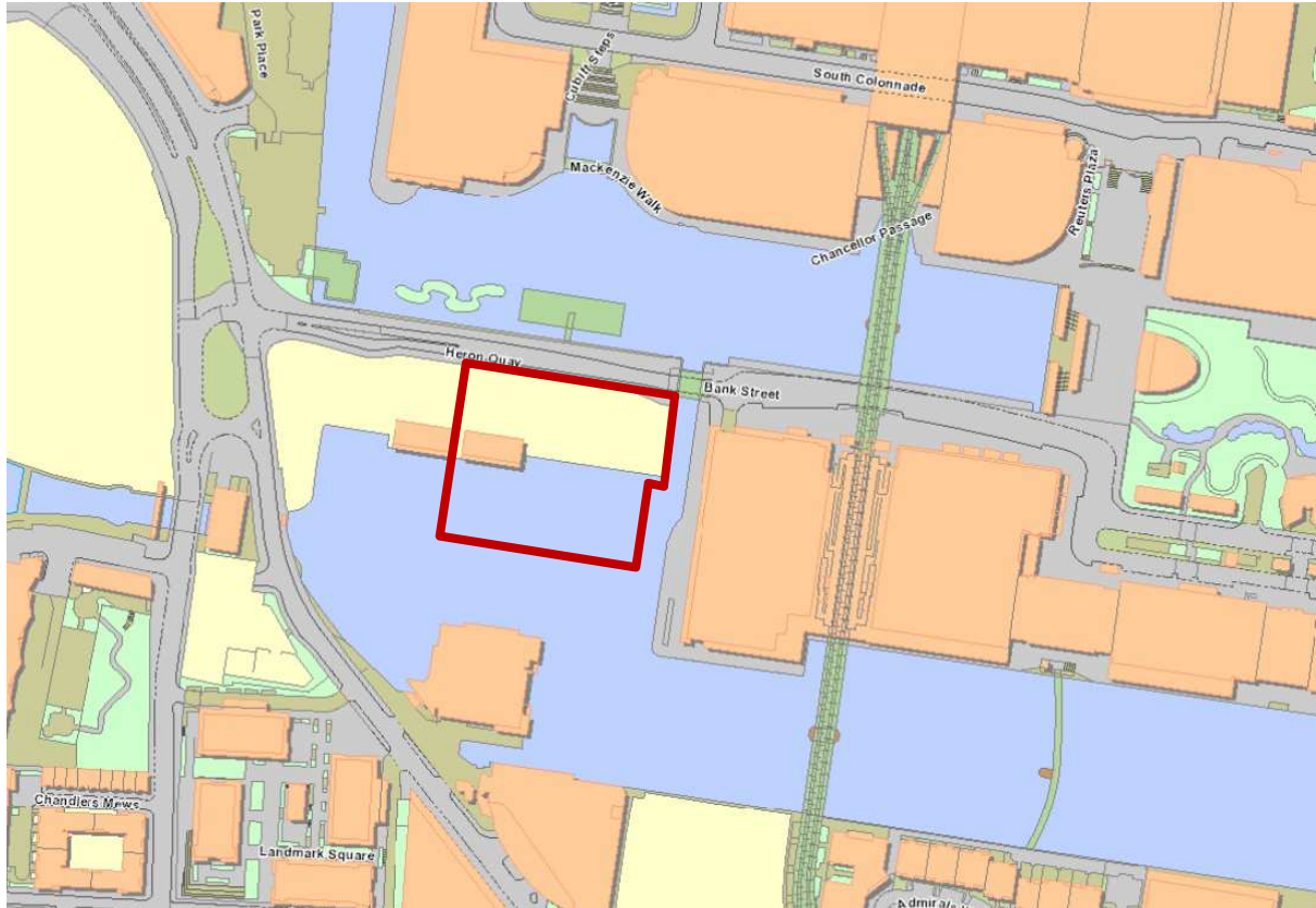
Figure 2 – Site location plan showing previous extent of dock, prior to construction of the cofferdam at the site and at 1 Bank Street, immediately to the west.
